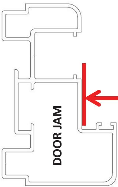
When measuring for a glass swing door, measure from the floor the top jamb like shown here and subtract  $\frac{3}{4}$ ". This will allow for a  $\frac{1}{4}$ " at the top and  $\frac{1}{2}$ " at the bottom. Be sure to check both sides and adjust accordingly.
