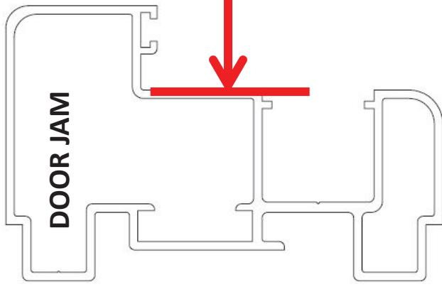
When measuring the width of the all glass swing door, measure from the two inside points shown above and subtract  $\frac{1}{2}''$ . For our standard width doors you should get  $35\frac{1}{2}''$  for a width.
