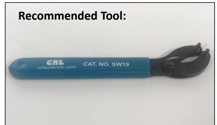
Adjustable Spanner Wrench for tightening Carriage Caps
