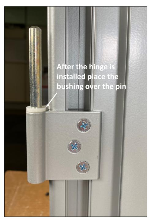
Attach the Hinge half with the Hinge Pins onto the Door Jamb. To attach, remove the preinstalled set screws from the Hinge Plate, align the holes of the Hinge to the Hinge Plate. Re-install the set screws. Tighten the set screws to hold the hinge in place. Exact location of the hinge will be set once the door is on the hinges.
