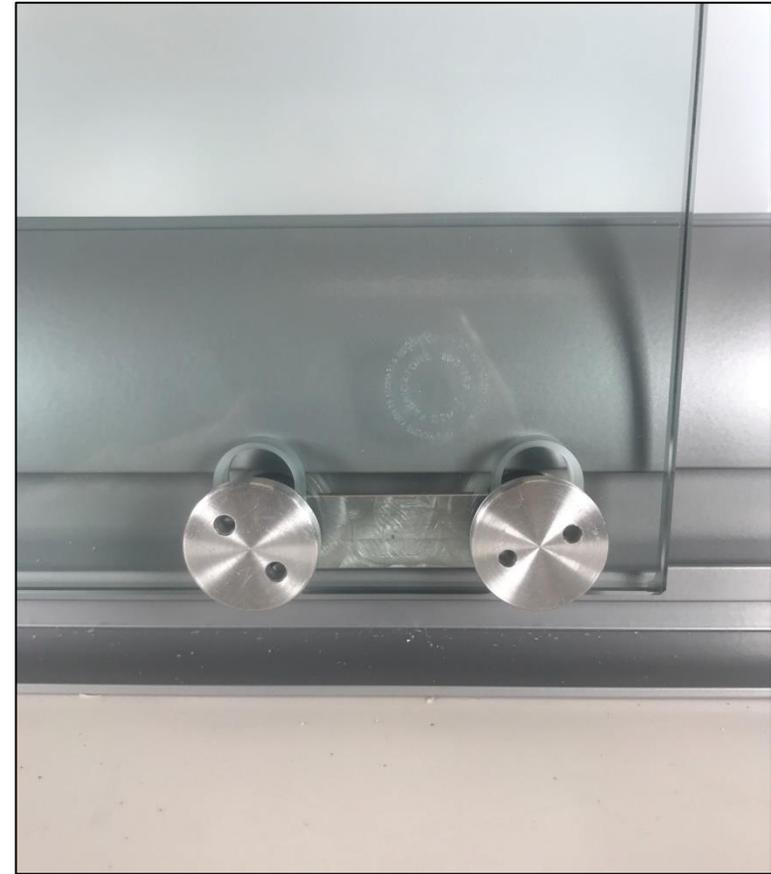
Install Carriage Caps with Washers onto the Carriage Frame. Center the Carriage within the Track and then tighten the Carriage Caps. The Carriage at the bottom of the door acts as the floor guide for the door.
