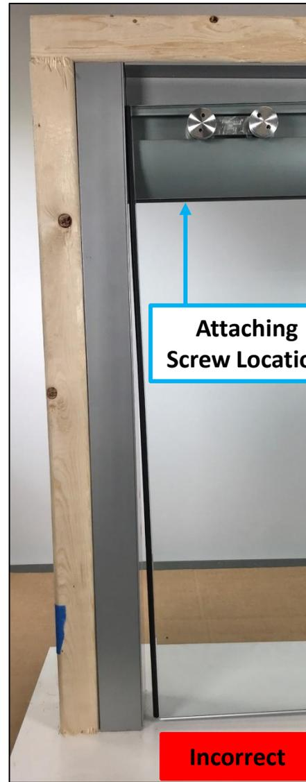
If there is an uneven gap between the framing and the door when the door is closed, adjust the attaching screw within the door opening to create tight and even gap.
