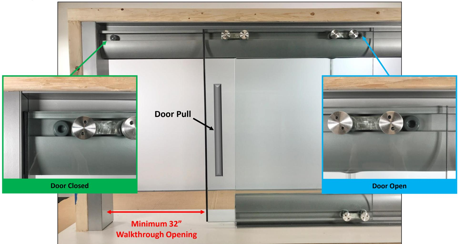
First, slide the door into its closed position. Next, place a Door Stop in front of the Carriage wheel within the View Track as shown above. Anchor the Door Stop with the provided screw. **Note:** Make sure the D-Pad is tight to the Wall-Start when determining the door stop location.
