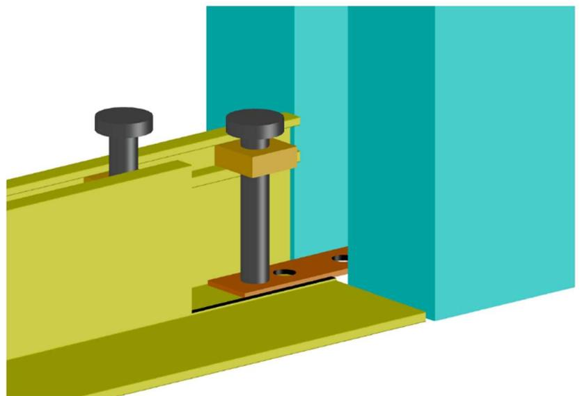
45. **Important Step:** Same as the ceiling adjust the Leveling Bolts in the View Guide. The Leveling Bolts must be level across the opening. Fig. 34.
